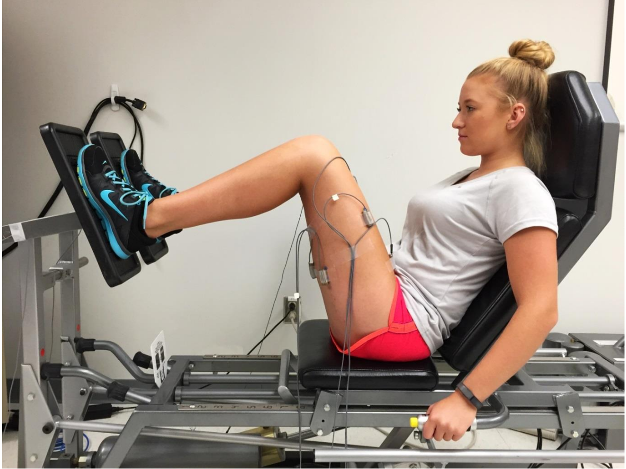
Figure 5.1: Subject positioned on the instrumented pneumatic leg press device for assessing lower extremity strength and power.
