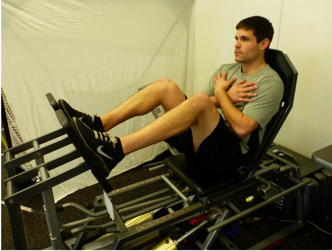
Figure 3.1: Subject positioned on Keiser A420 pneumatic instrumented leg press device for measuring lower extremity strength and power.
