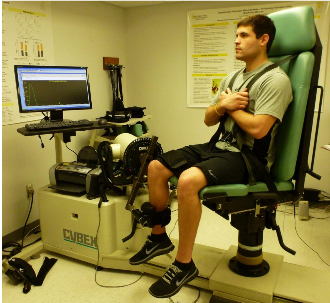
Figure 4.1: Subject positioning for isometric testing of quadriceps muscle strength and RTD and for training with high intensity voluntary isometric knee extension contractions.
